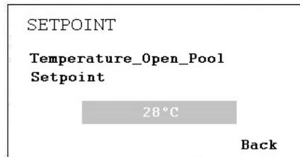
Push the **Rotate button** and you can now change the value by turning the **Rotate button** and then push the button again. Now the set point is changed.
