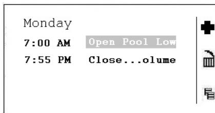
To activate the three icons on the right side of the display you have to press the button on the controller which is beside the icon. The three icons are having the following functions:
