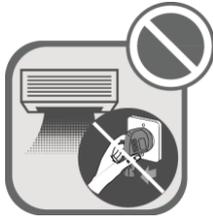
Never start or stop the air conditioner by inserting or removing the power cord.
