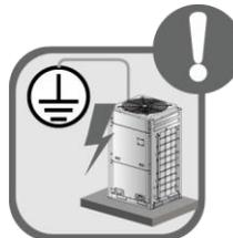
This air conditioner must be properly grounded through the receptacle to avoid electric shock. The grounding wire shouldn't be connected with gas pipe, water pipe, lightning arrester or telephone line.
