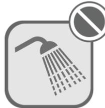
Do not spray water on the air conditioner or it will cause malfunction or electric shock.
