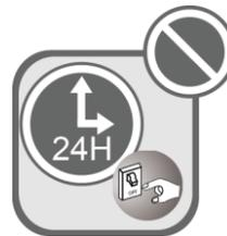
Connect power supply 8 hours before operation. Do not disconnect power if you want to stop the unit in a short period of time, e.g. in one night. (This is for protecting the compressor.)
