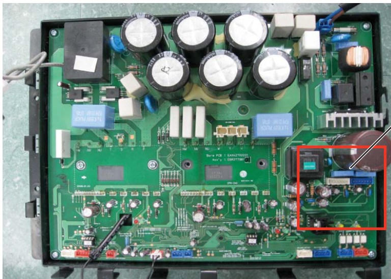
<FAN Motor Connection check>
