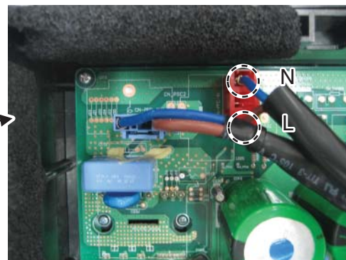
< Main PCB wiring Check Point >
