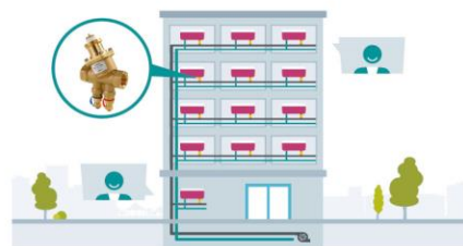
Dynamic hydronic balancing: The hydronic system is always balanced, independent of load conditions and pressure fluctuations.
